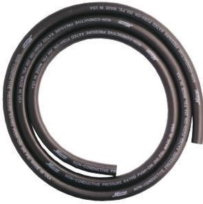
Made of strong, flexible Nitrile with spiral synthetic yarn reinforcement. Resists oil, gasoline, abrasion and ozone. Highly resistant to petroleum based hydraulic oils. No clamps or ferrules needed, just cut hose to desired length and push on fitting. Ideal for automotive paint shop, construction, manufacturing and petrochemical industries. Use with compressed air, water and petroleum based solvents. Fittings are not included with bulk push and lock hose
