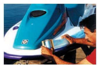
21" for masking along edge of jet ski between hull top and bottom
