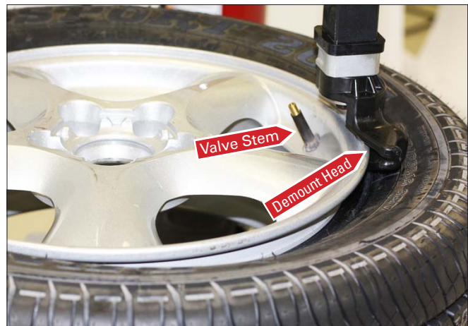
Figure 17 - Position Valve Stem Behind Demount Tool Tail
