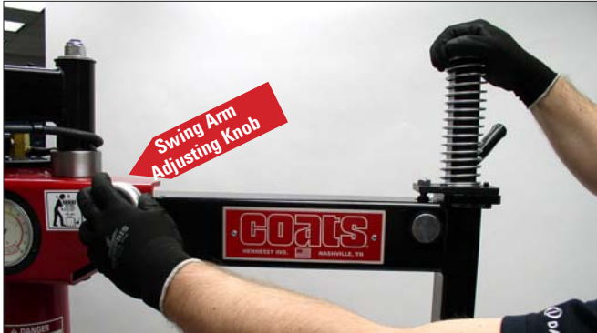
Figure 8 - Adjust Swing Arm to Position Tool Roller
