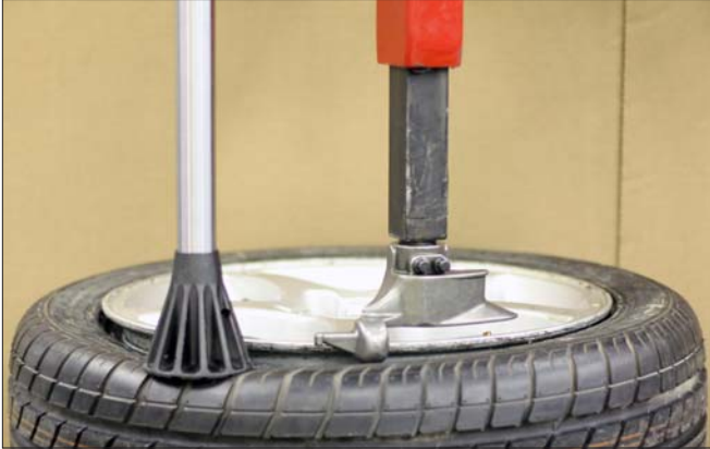
Figure 14 - Robo-Arm LR Foot Depressing Sidewall of Tire
